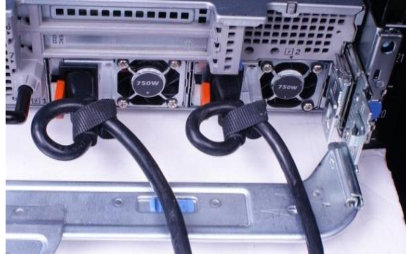
Figure 2. Routing power cables through the strain reliefs
