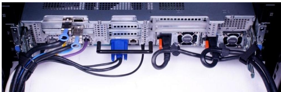
Figure 9. Cable routing without a CMA
