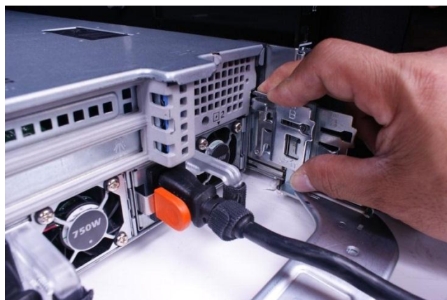
Figure 3. Attaching the inner CMA attachment bracket
